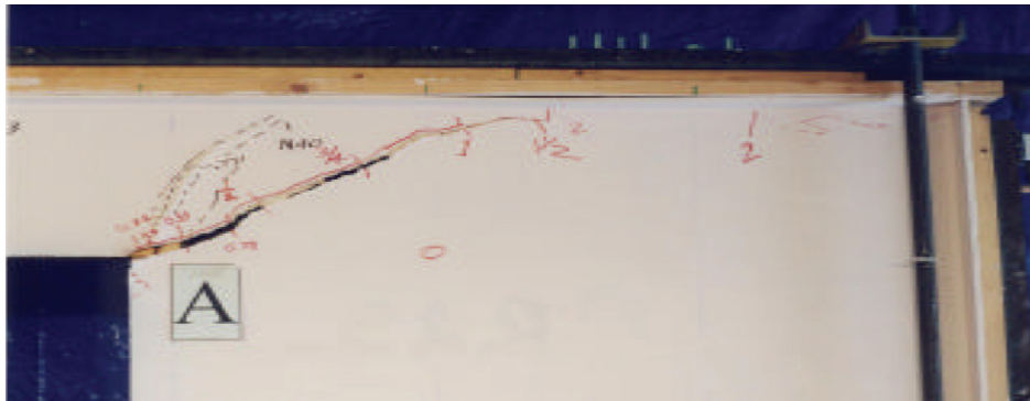
Figure 2 - Damage State 2 for Partition Walls with Gypsum Wallboard: Global/or Local Buckling and Crushing of Wallboard (from McMullin et al. 2001).
