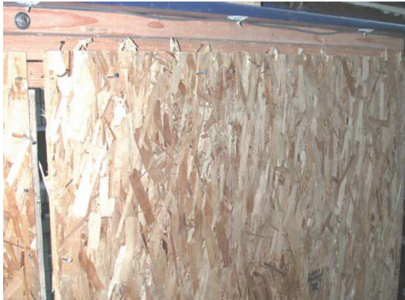
Figure 5 - Damage State 2 for Walls with OSB/Plywood Sheathing (System #50): Replacement of OSB/Plywood (from Gatto and Uang 2002).
