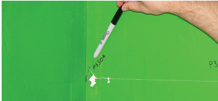
Figure 1 - Damage State 1 for Partition Walls with Gypsum Wallboard: Dimpling of Wallboard over Nail/Screws, Cracking at Vertical or Horizontal Seams (from Christovasilis et al. 2007).
