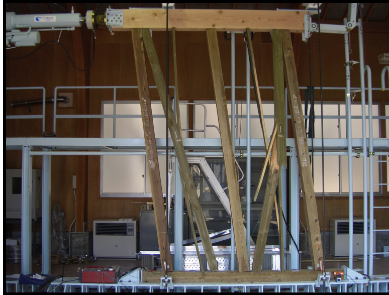
Figure 14 - Damage State 1 for Wood Stud Framing Braced by Diagonal Bracing: Failure of Diagonal Bracing (from Isoda 2007).
