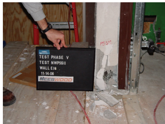
Figure 10 - Damage State 2 for Walls Incorporating Stucco as Exterior Finish: Replacement of Spalled Stucco (from Christovasilis et al. 2007).
