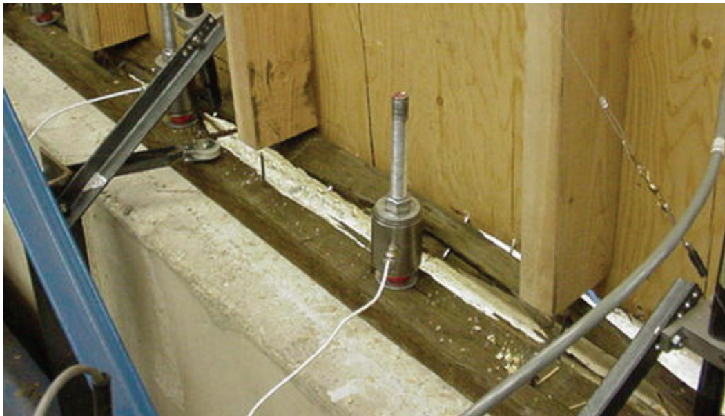
Figure 17 - Damage State 1 for Sill Plates without Holdowns: Replacement of Entire Wall (from Mahaney and Kehoe 2002).
