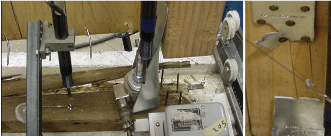
Figure 20 - Damage State 1 for Sill Plates with Holdowns: Replacement of Entire Wall (from Mahaney and Kehoe 2002).
